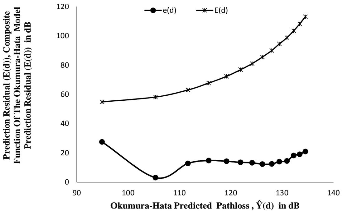
**Figure 2.** Graph of prediction residual ( $e(d)$ ), composite function of the Okumura-Hata model prediction residual ( $E(d)$ ) versus Okumura-Hata predicted pathloss ,  $\hat{Y}(d)$
