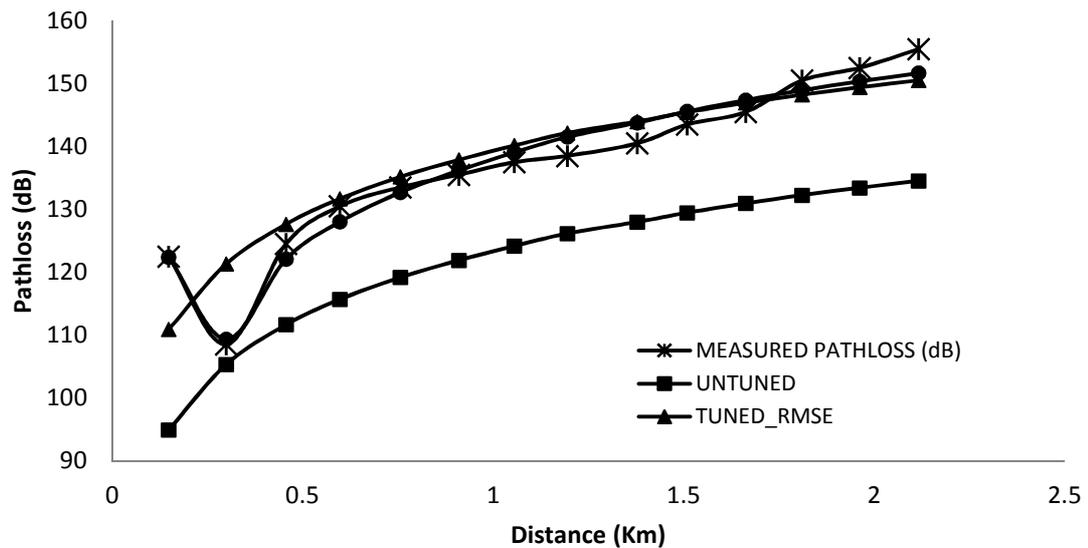
**Figure 2.** Tuned and Untuned Pathloss Versus Distance
