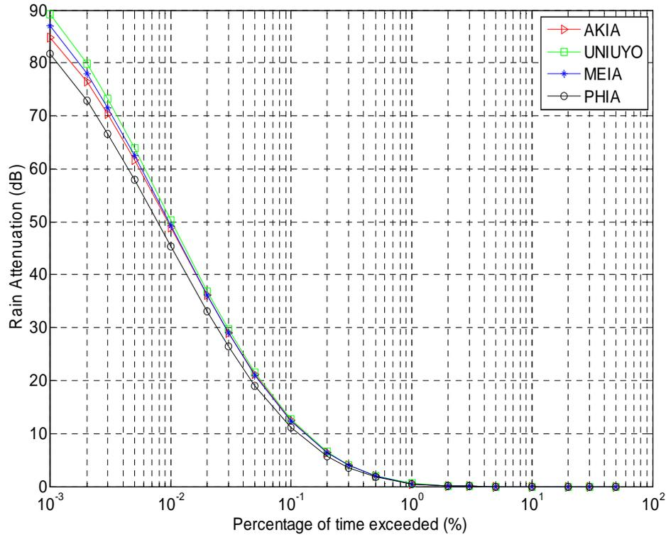
**Figure 2.** Cumulative distribution of rain attenuation at 20 GHz
