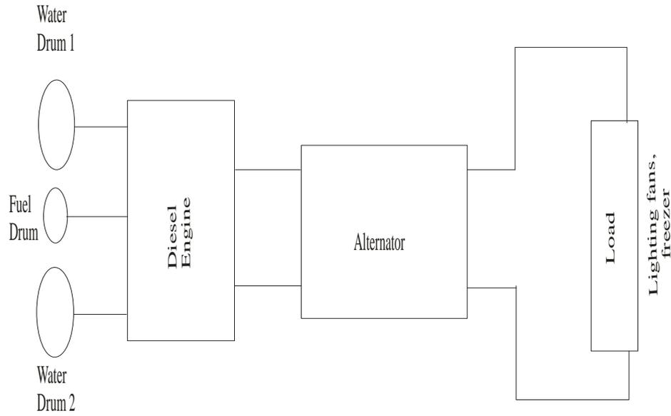
**Figure 4:** Schematic diagram of the conventional diesel power plant used in most Nigerian households.
