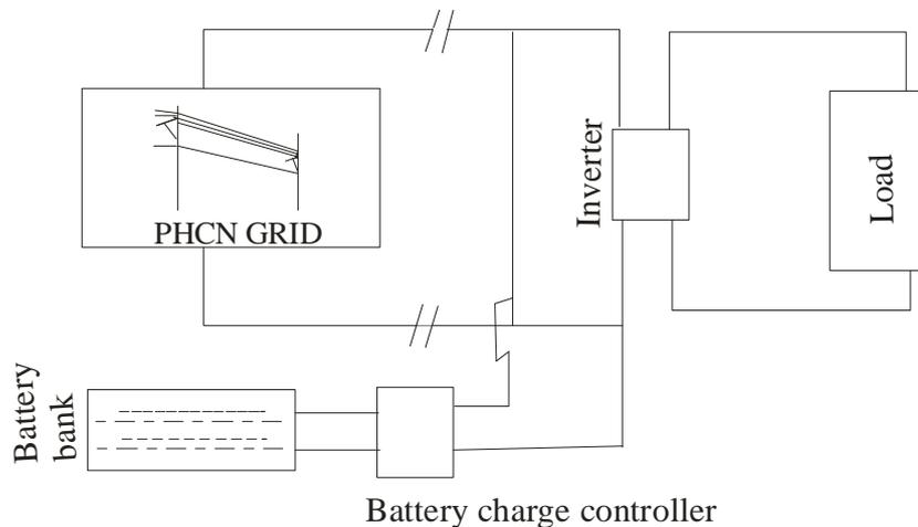
**Figure 1:** Schematic diagram of the Battery back-up system in use in most household in Nigeria.
