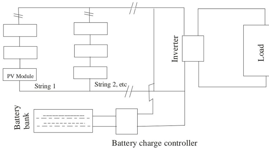
**Figure 2:** Schematic diagram of a stand-alone photovoltaic power plant for use in Nigeria household
