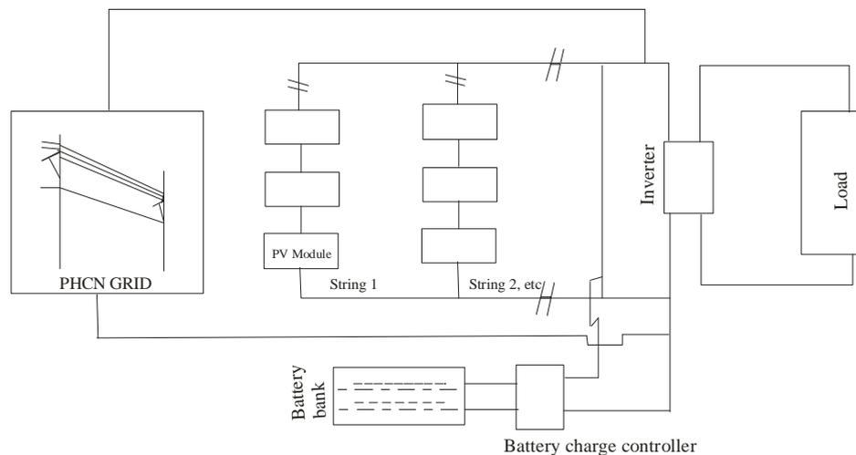
**Figure 3:** Schematic diagram of a hybrid photovoltaic power plant for use in Nigeria Household
