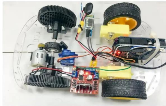
Figure 4. An example implementation of a cart programmed with Arduino [3].
