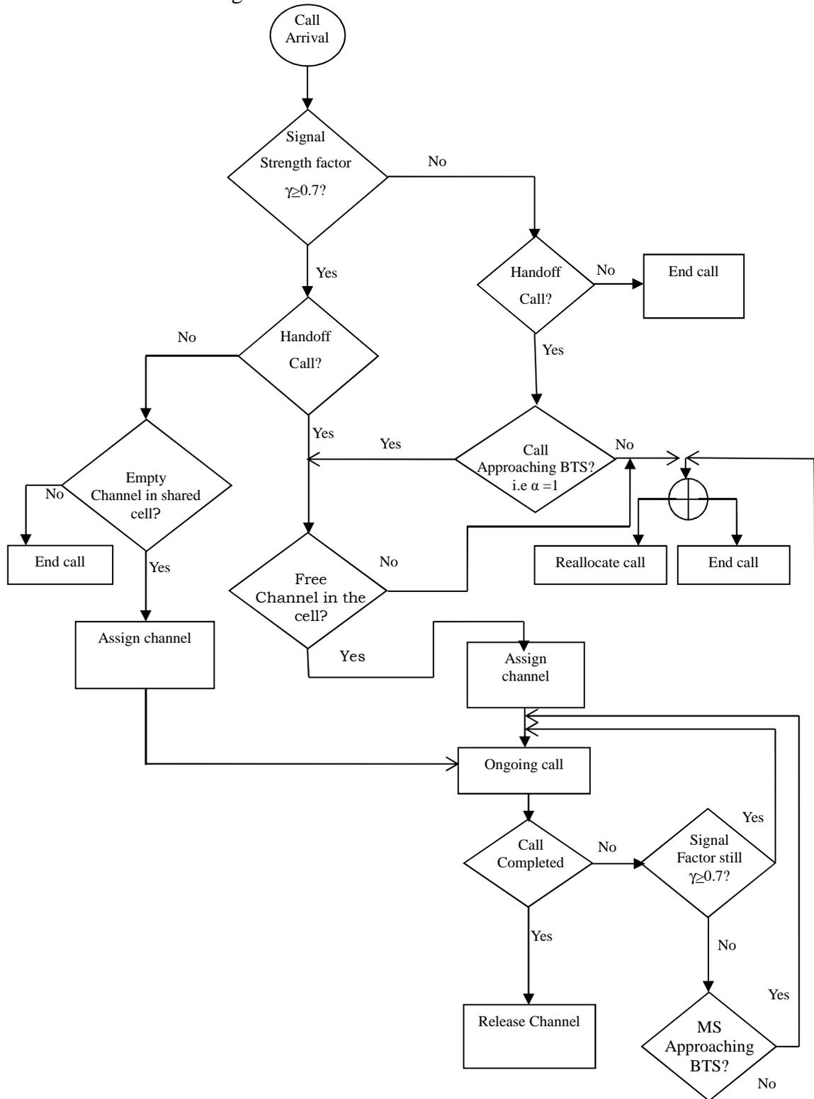
Figure 2: Schematic flowchart of the new scheme
